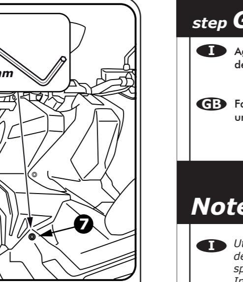
**GB** Fasten the leg cover on both sides, using the scooter's original screws, threading them through the holes at point 7.
