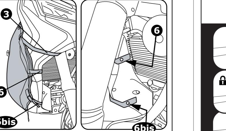
**GB** Fasten Termoscud® on both sides, using the scooter's original fasteners\*, threading them through the holes at the end of the straps 6 and 6bis.
