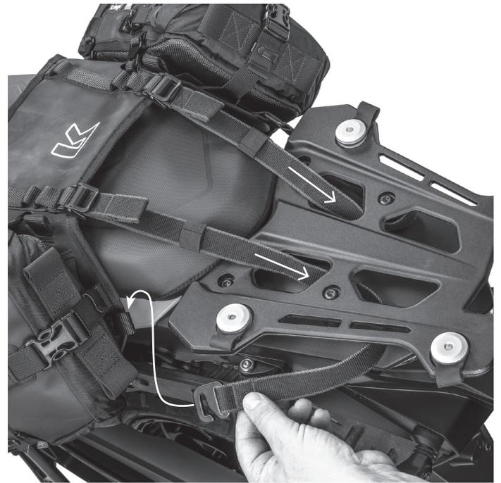
**2** Set the top straps to the longest length and slide the elastic loop near to the buckle. Pass a top strap down through the opening on the baggage carrier and around the rear alloy spacer and hook to the web loop, with the hook pointing down. Repeat on the other side.
