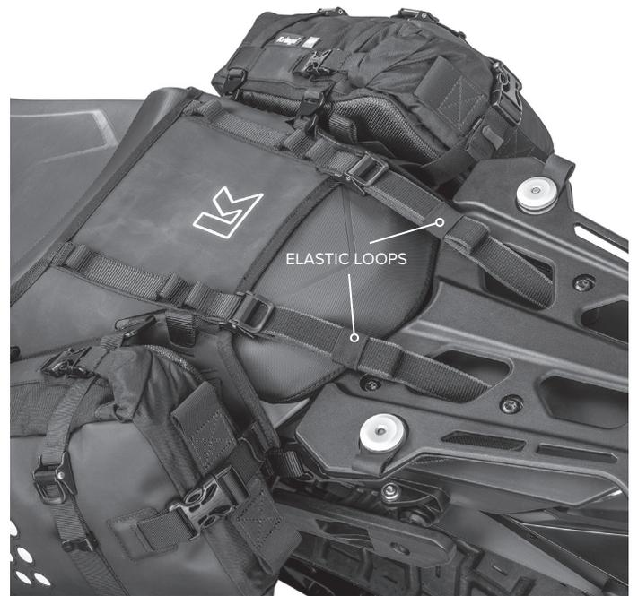
**4** Once the OS-BASE is tight on the seat, fold over the loose strap ends and place them in the elastic loops.
