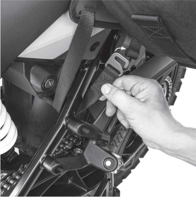
**1** Lay the OS-BASE over the motorcycle seat, forward from the final fitting position. Pass the front hook strap under the cross member on the frame and attach the hook to the web loop so the hook is pointing down. Repeat on the other side.
