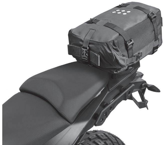
To fit, remove the KTM baggage carrier. Add thread lock to the 25mm M6 screws and insert from the underside. Mount the KTM Rack-loops as shown in the diagram.
