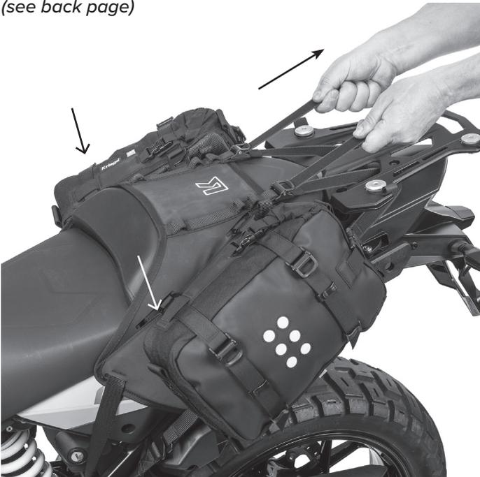
**3** Standing at the rear of the bike hold both loose straps ends and pull until the OS-BASE is firmly mounted on the seat. A strong tap downwards on each OS-PACK will help the OS-BASE slide further onto the seat.
